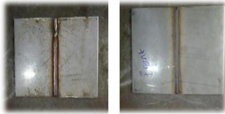
Figure 2: (a) SMAW process (b) TIG process.
