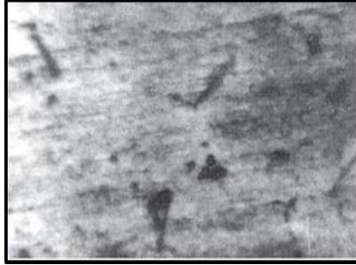
Figure9: Optical micrograph of TIG welding at high heat input (100 x).
